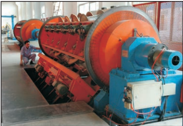
Individual motor control strander with side bottom loading device
