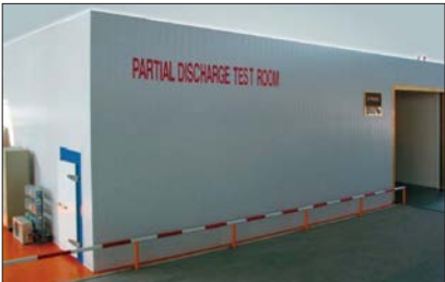
Shielded room for 220kV cables(High Volt equipments)
